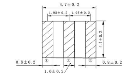
Connection: (1) Input (2) Ground (3) Output
