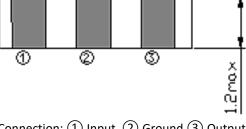
Connection: (1) Input (2) Ground (3) Output
