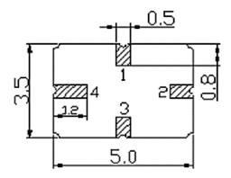
PIN NO.CONFIGURATION1Input/Output3Output/Input2, 4Case Ground
