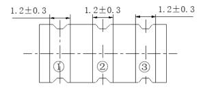
Connection: 1 Input 2 Ground 3 Output
