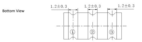
Connection: (1) Input (2) Ground (3) Output
