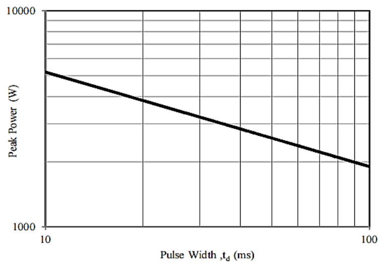
Fig. 4 - Peak Pulse Power Rating Curve
