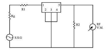
Rg + R1 = R2 = Input/Output Impedance
