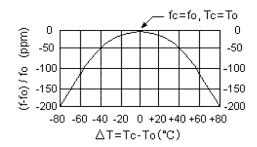
Note: The curve shown above accounts for resonator contribution only and does not include LC component temperature contributions.
