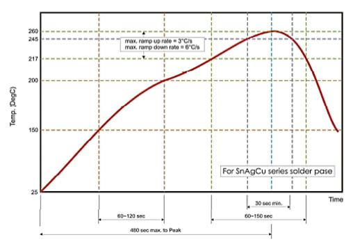
Fig 2. Infrared soldering profile for Chip Resistors
